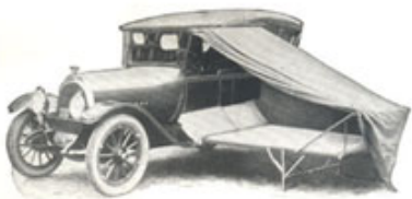
How the same running-board outfit looks when unpacked and set up. The tent is drawn aside to show the construction of the bed.
