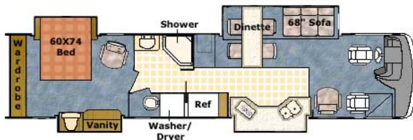
Figure 29. Floorplan of a Quadruple-Slide Class A Motorhome
